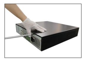
Figure 1-23 Install the cover and screws
