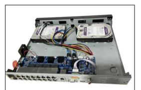
Figure 1-19 Fix the HDD
