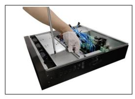
Figure 1-22 Fix the HDD
