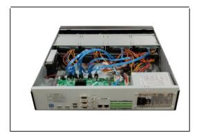
Figure 1-21 Connect the power and data cables
